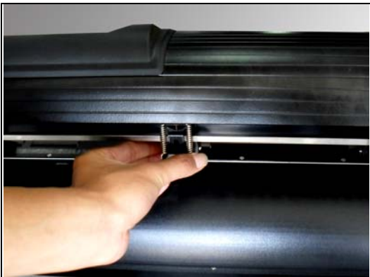
Figure 4-3 correct way to move pinch rollers
